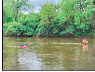
Hydrologist Aleia Couchman collects water quality sample at Yellow R. at Knox on May 23, 2024, while ADCP equipment is being prepared to conduct a discharge measurement. Photo taken by Madelyn Messner.
